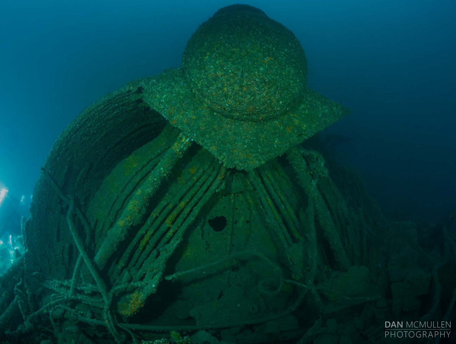
Figure 35: The 1 st "Normand" boiler on the bow section of Tiger with the distinctive three-drum design consisting of a steam drum above two water drums in a triangular layout, with water tubes filling in the two sides of the triangle. Photo credit: Dan McMullen.
