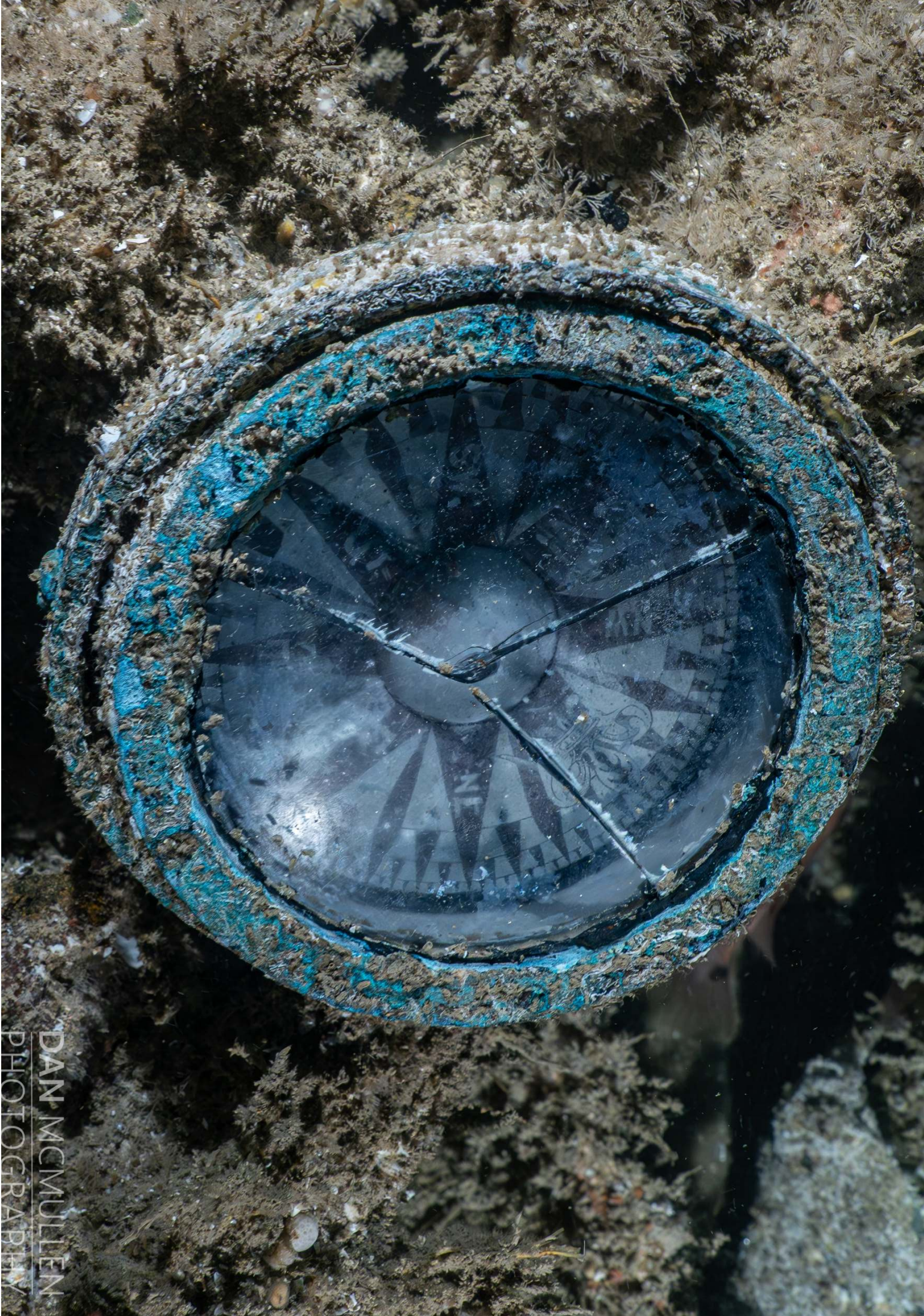
Figure 17: A Dent & Co. London fluid compass with a 128-point graduated card and fleur-de-lis pointing North. Photo credit: Dan McMullen.
