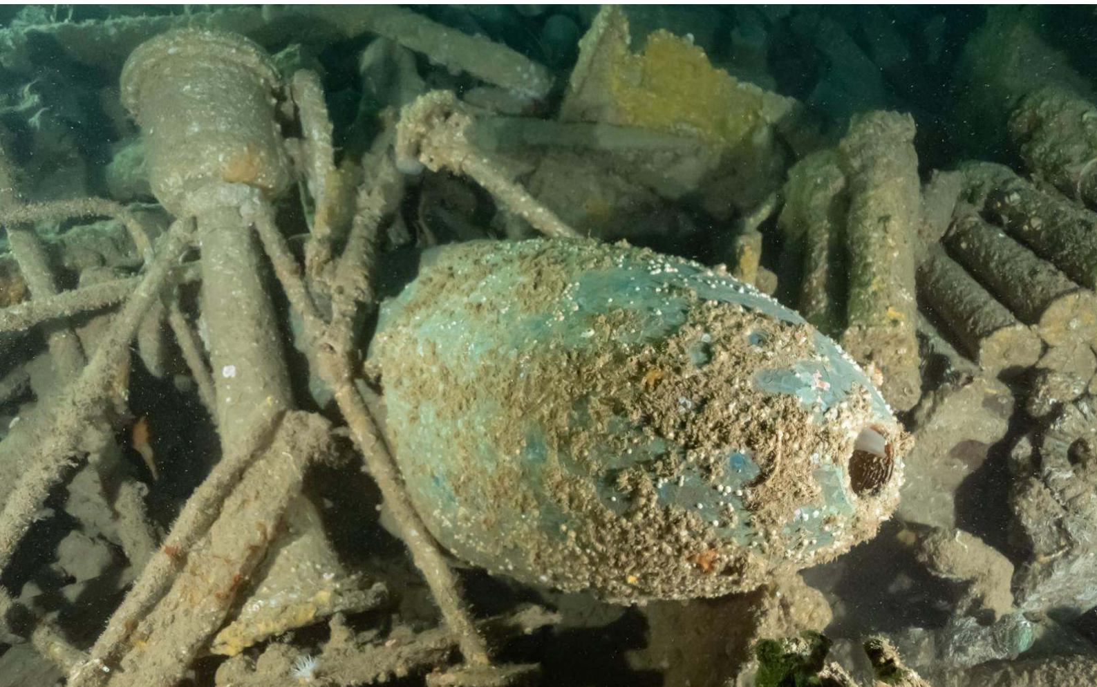
Figure 31 (below): The head of an 18-inch Whitehead torpedo with a threaded hole ("pistol socket") in the torpedo nose measuring approximately 55mm (2.1 inches) in diameter for fitting the "pistol" that triggered the main explosive charge. Photo credit: Joe Colls Burnett.
