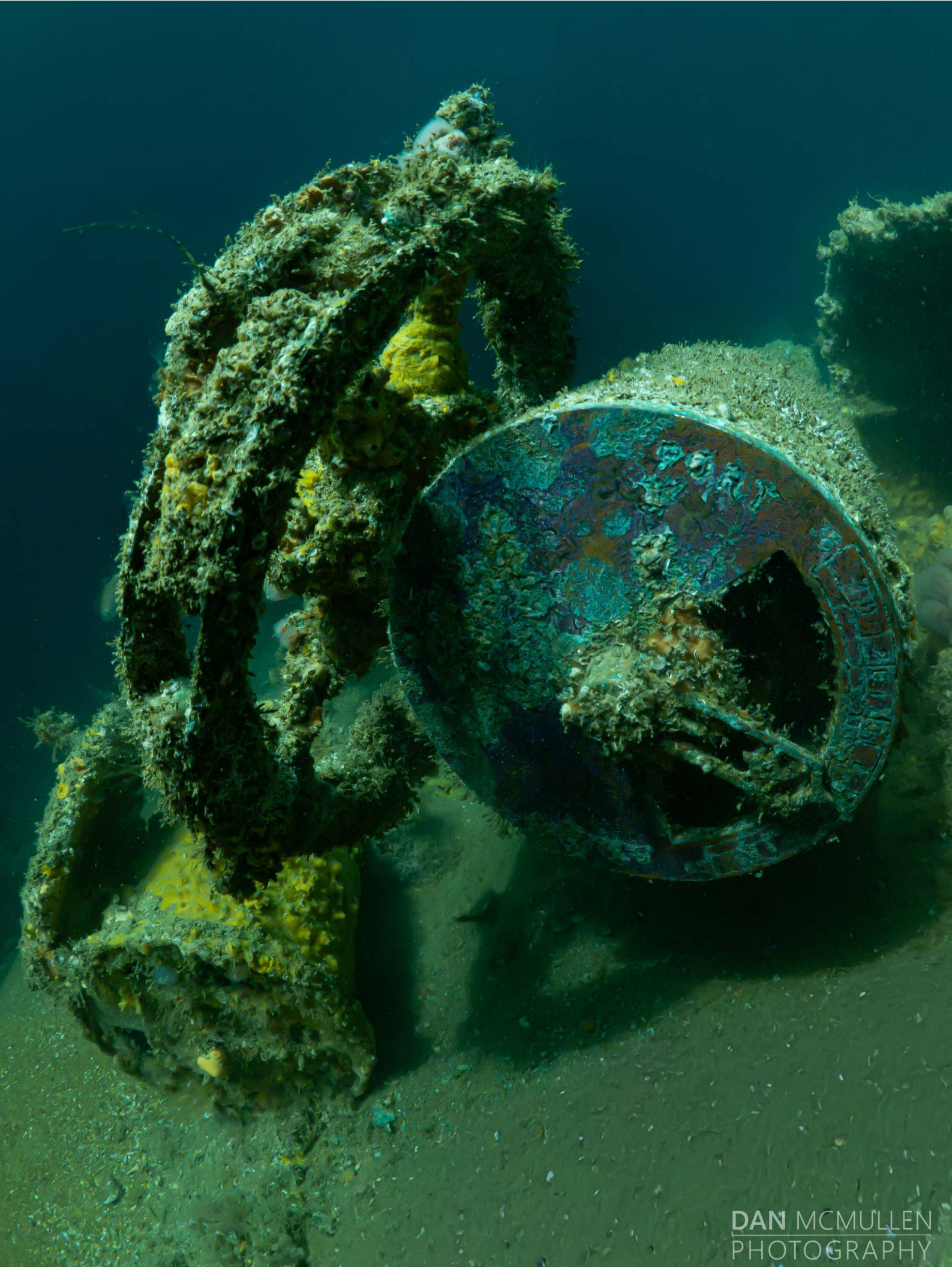
Figure 34: The rudder position indicator. The graduated circular scale is marked "PORT" and "STARBOARD". The pointer mechanism is set to approximately 5-10 degrees to starboard, which suggests that Tiger had not altered course to avoid Berwick immediately prior to the impact. Photo credit: Dan McMullen.
